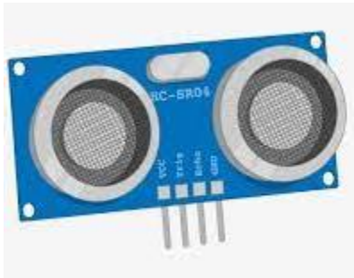
Figure. 4. Schematic view of Ultrasonic water level sensor.
